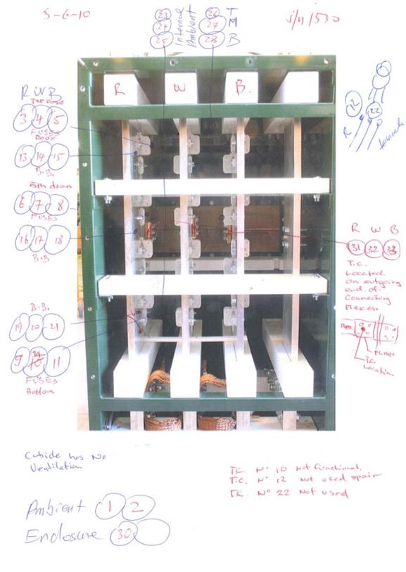
Fig 13 – Temperature Rise Measurement Points
