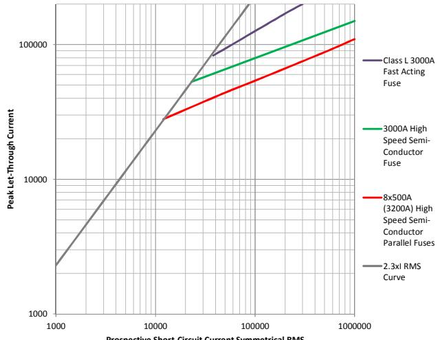
Fig 4 – Peak Let-Through Comparison between a single Class L 3000A, a HSSC 3000A and 8 x 500A (3200A) parallel HSSC Fuses
