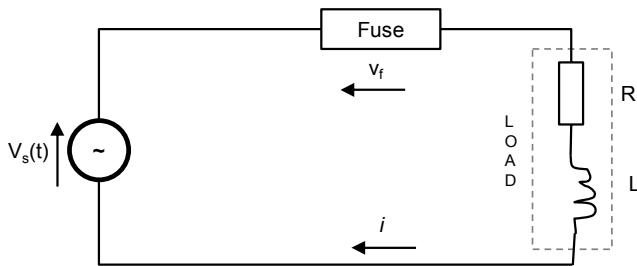
Fig 1 - Equivalent Circuit of Fuse and Connected Load
