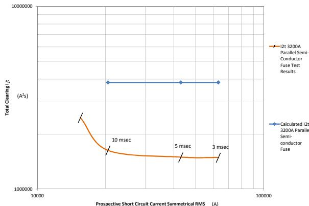
Fig 11 – 8 x 500A  $I^2t$  Characteristics
