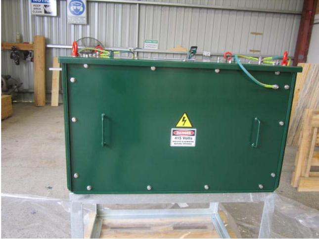
Fig 30 – 500KVA IP56 Module - 2012
