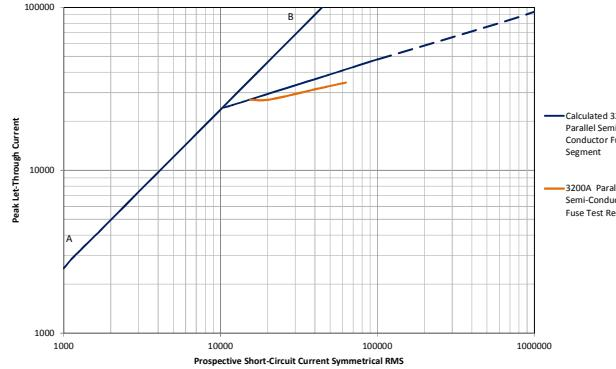
Fig 8 – 8 x 500A Interrupter, Peak Let-through, Calculated vs Test Clearing Time
