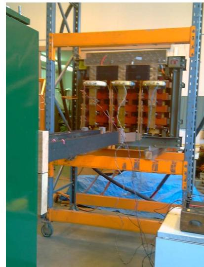
Fig 12 – Temperature Rise Current Injection Test Rig
