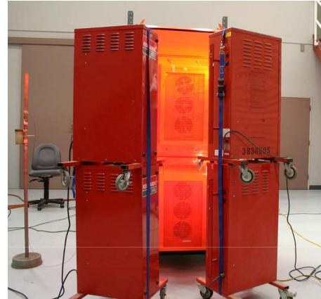
Fig 17 – IP56 Module Undergoing Extended Temperature Rise Test
