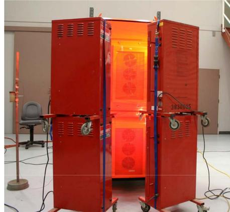
Fig 17 – IP56 Module Undergoing Extended Temperature Rise Test
