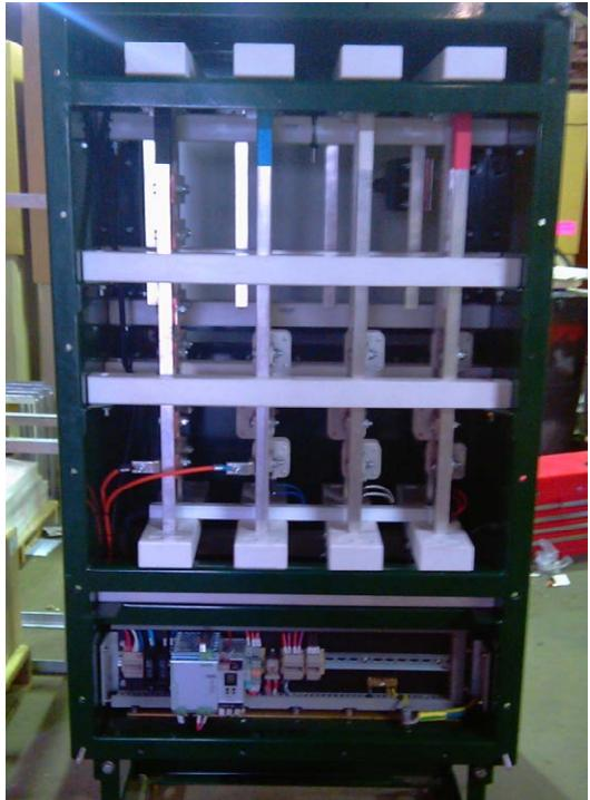
Fig 26 – Prototype 750kVA Forced Cooled Module – 2010
