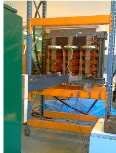
Fig 12 – Temperature Rise Current Injection Test Rig
