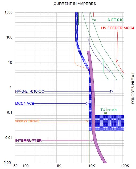
Fig 23 – MCC TCC with Interrupter Mitigation and 500kW DOL Motor Start
