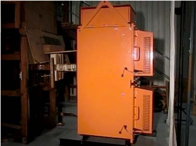
Fig 19 – IP56 Module Undergoing Arc Fault Containment Test, TUV Rheinland Test Report No 19300582004
