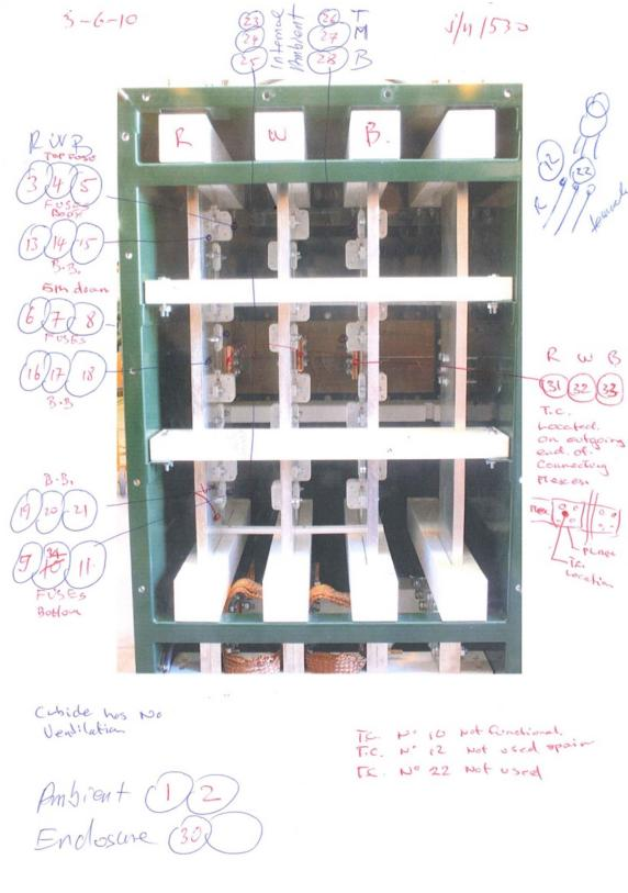
Fig 13 – Temperature Rise Measurement Points
