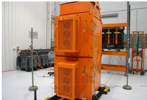
Fig 15 – IP56 Module Undergoing Temperature Rise Test
