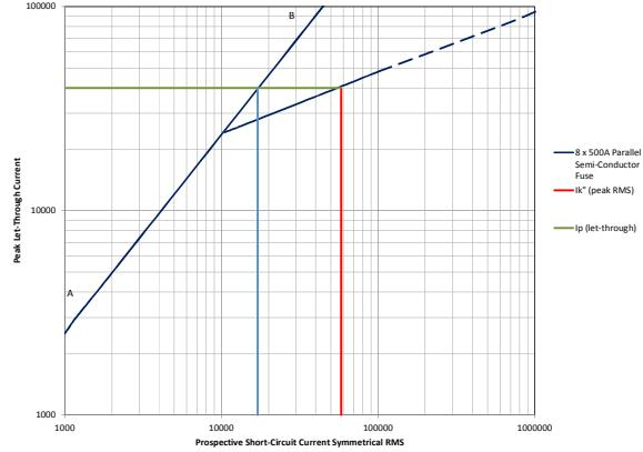
Fig 22 – MCC4 prospective fault current after Interrupter's are installed
