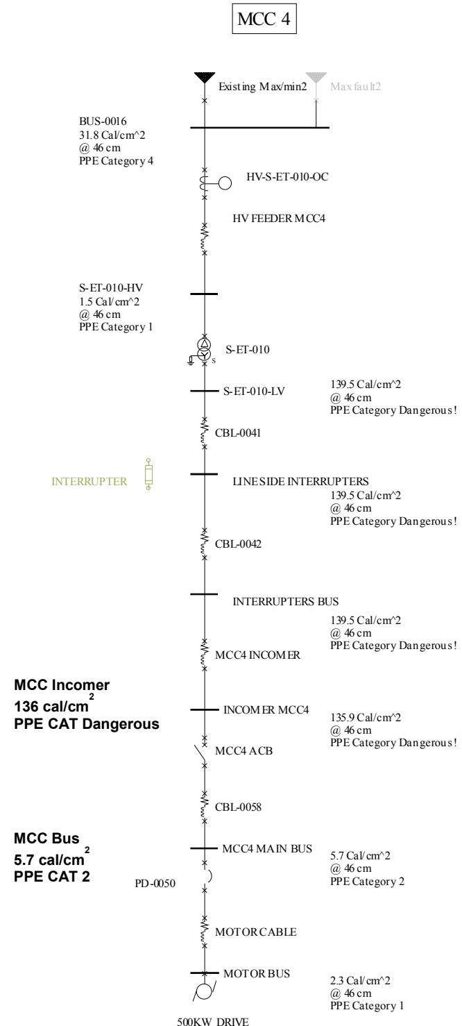
Fig 20 – Software One Line with no Interrupter Mitigation
