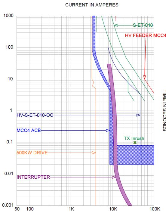
Fig 24 – MCC TCC with Interrupter Mitigation and 500kW VVVF Motor Start
