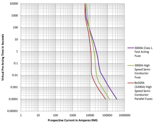
Fig 3 – TCC Comparison between a single Class L 3000A, a HSSC 3000A and 8 x 500A (3200A) parallel HSSC Fuses
