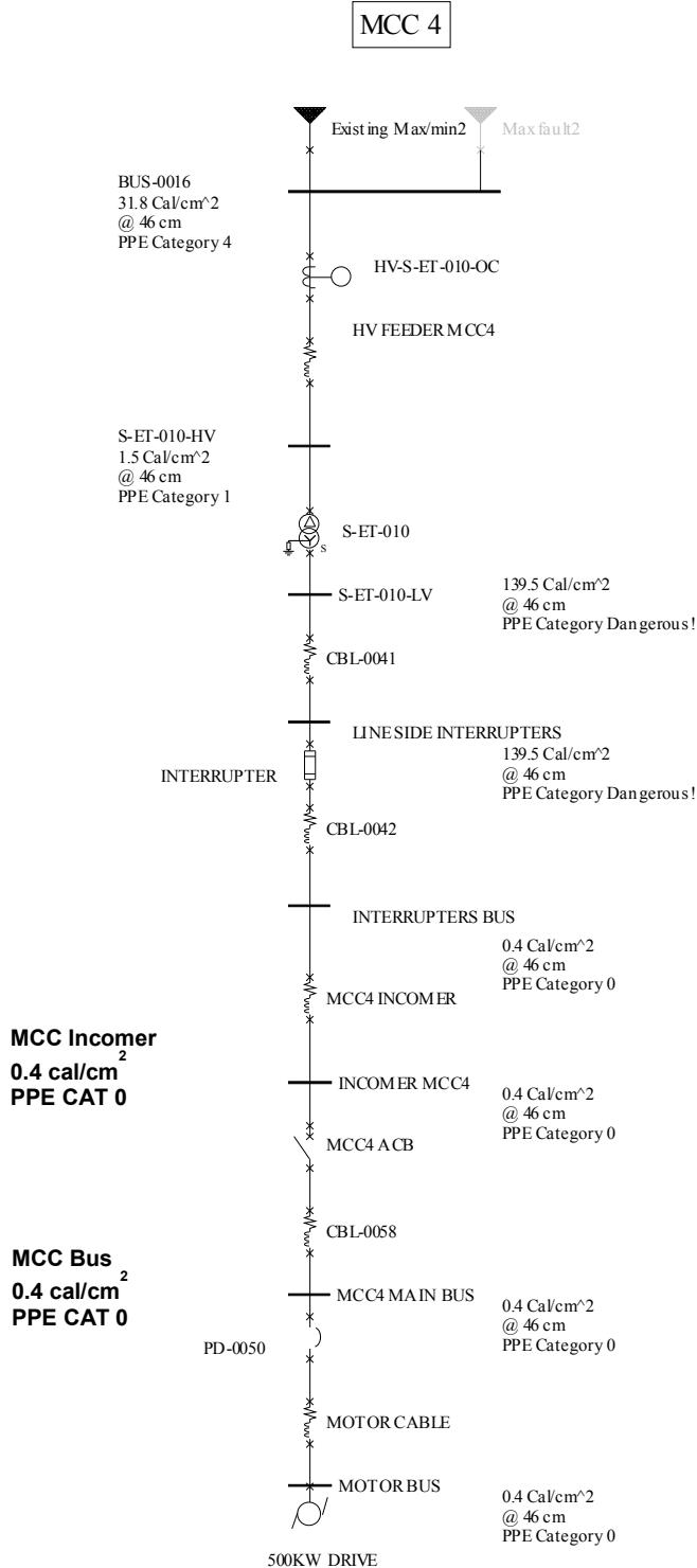
Fig 21 – Software One Line with Interrupter Mitigation
