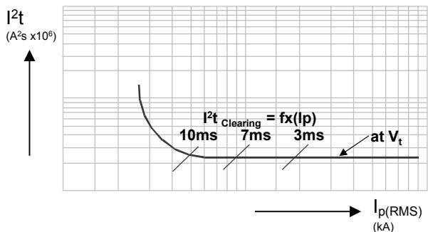
Fig 5 – Typical  $I^2t$  Characteristic Curve Showing Constant Let-Through Energy in the Current Limiting Range
