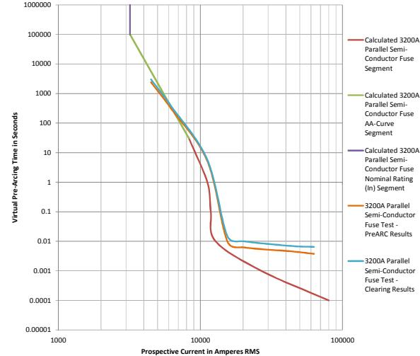
Fig 9 – 8 x 500A Interrupter Time Current Curve, Calculated Pre-Arc vs Test Clearing Time
