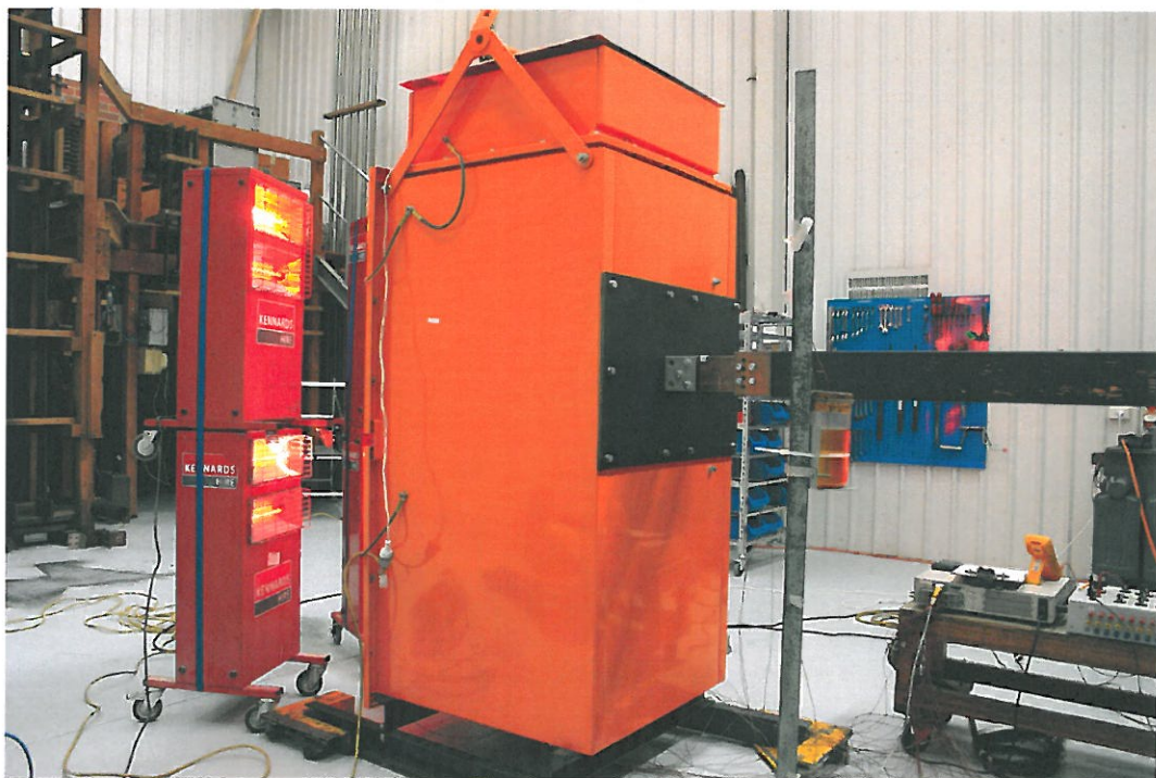
Photo 12619: Back of Assembly with Heaters in Place
